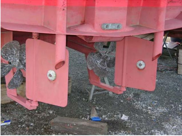
Anodes are typically made from Zinc, Aluminium, Magnesium or mixed alloys. Zinc is in widespread use in salt waters, but cannot protect yachts that have either aluminium hulls or with aluminium fittings, such as sail-drive or stern drives units.
