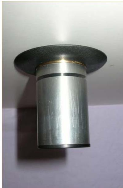
The unique cone connection design allows use of a low strength nylon screw whilst retaining excellent electrical and mechanical contact.
