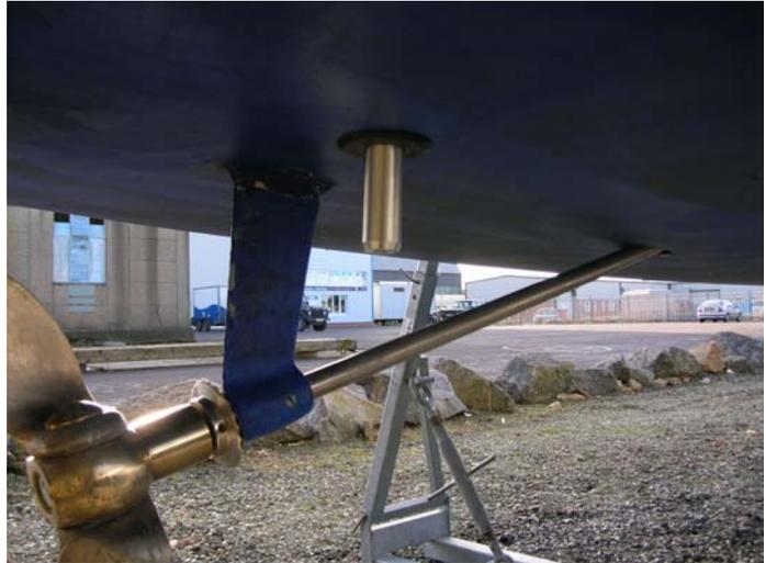
Plastic, stainless steel and bronze skin fitting options, all with proven record for safe through hull installations are available to make **IonGuard** suitable for all hull types including wooden, steel, aluminium, ferro, GRP and all new laminate and composite hull types.
