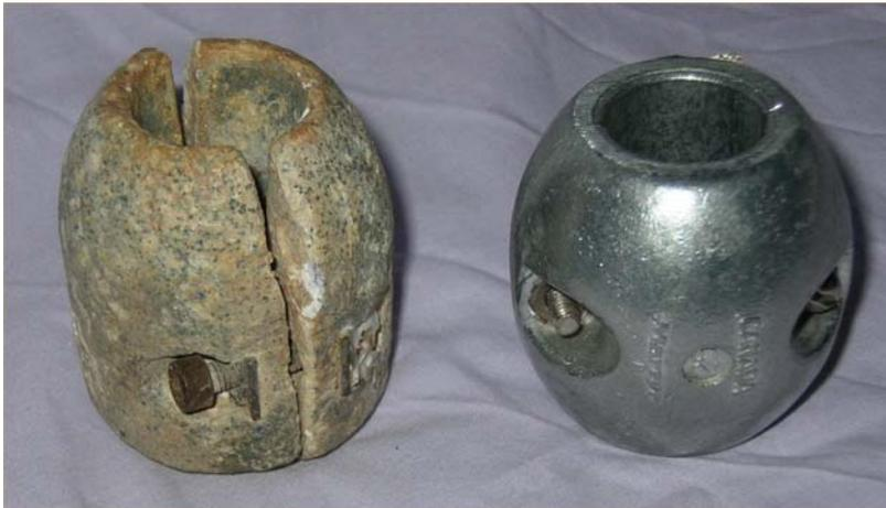
The zinc anode pictured on the left has only been immersed for a few months in brackish water yet has collected a thick non-reactive oxide coating, rendering the anode useless for cathodic protection.
