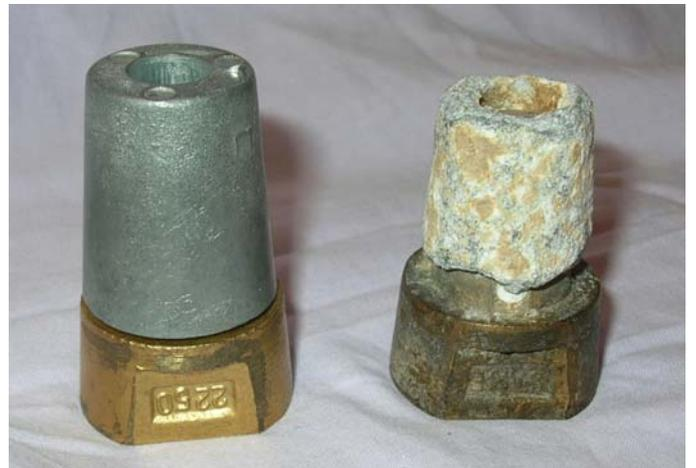
applications and if used on a boat in salt water, the very low voltage causes the formation of hydrogen bubbles that often results in the paint being stripped from aluminium parts in just a few hours followed by rapid corrosion.
